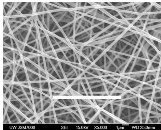
**Figure 2** Result of concentration experiment showing 60/40 PCL/chitosan nanofibers. Scale bar is 10  $\mu\text{m}$ .
