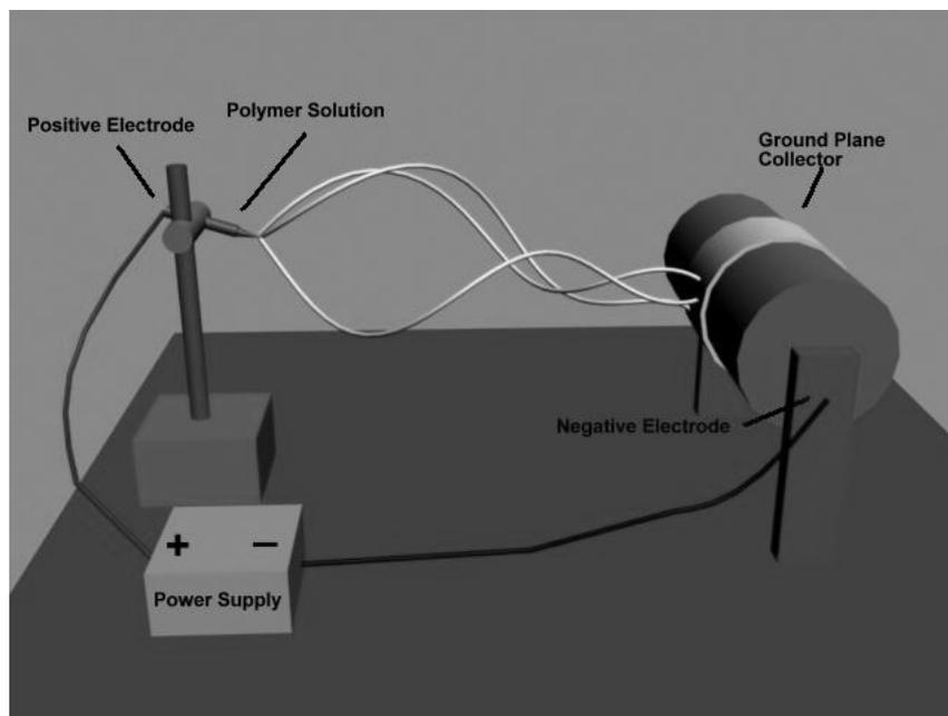
**Figure 1** Typical electrospinning setup.
