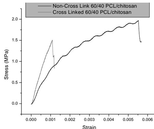
**Figure 3** Tensile test revealing breaking strength, elasticity, and Young's Modulus for both crosslinked (thin) and non-crosslinked (thick) fibrous mats.
